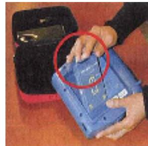
4. Press the top end down until the battery clicks into place.
