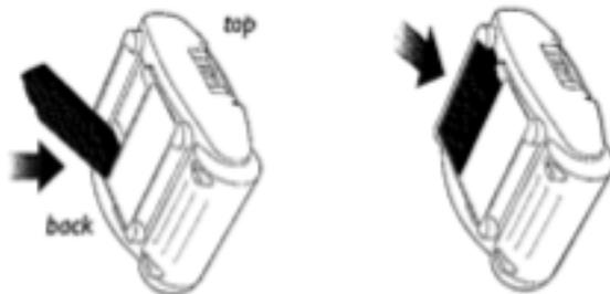
6. Press the top end down until the battery clicks into place.
