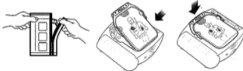
5. Insert battery back into AED. Put the battery, bottom end first, into the battery compartment on the back of the AED
